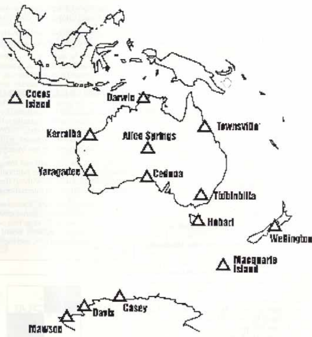
Figure 8 - The Australian Fiducial Network (AFN): permanent, on-line regional GPS station
